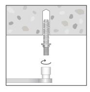
Insert anchor into hole and screw in using spanner, socket or an impact wrench. Apply constant forward pressure when driving and tighten to the specified torque.
