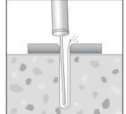
Clear hole of drilling debris.
