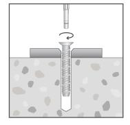
Insert anchor into hole and screw in using hand or power tool to drive Torx driver bit. Apply constant forward pressure when driving and tighten to the specified torque.
