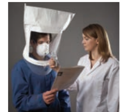
Pass or fail test that relies on the wearers ability to respond to an atomised liquid
