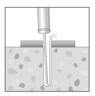
Clear hole of drilling debris.
