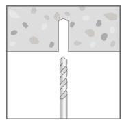
Drill hole into substrate to the specified diameter and depth.
