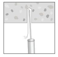
Clear hole of drilling debris.
