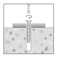
Insert anchor into hole and screw in using hand or power tool to drive Torx driver bit. Apply constant forward pressure when driving and tighten to the specified torque.
