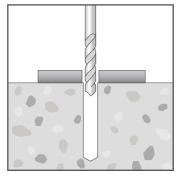
Drill hole through fixture into substrate to the specified diameter and depth.
