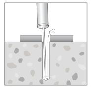
Clear hole of drilling debris.
