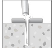
Clear hole of drilling debris.
