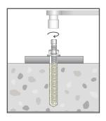
Once the cure time has elapsed, place the fixture and clamp it down using a wrench to tighten to the specified installation torque.
