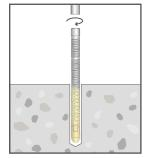
Using a power tool and the driver bit supplied with the studs, rotate & drive the anchor stud into the capsule until the anchor stud bottoms out in the hole. Stop driving and remove tool / driver at this point. PROTECT THE ANCHOR FROM DISTURBANCE UNTIL THE CURE TIME HAS ELAPSED.
