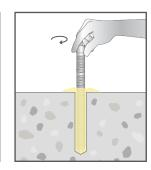
Ensure the anchor stud is clean and free of contaminants, grease etc. Push the anchor stud into the adhesive - slowly rotating the stud until it is seated against the base of the hole. An excess of adhesive around the top of the hole indicates sufficient material was injected into the hole, otherwise remove the anchor stud and renew the hole with adhesive.
