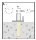
All steps prior must be completed within the working time of the adhesive. Protect the anchor from disturbance until the full curing time has been reached. Once full cure is achieved, carefully place the fixture and apply the specified installation torgue.
