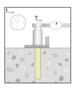
All steps prior must be completed within the working time of the adhesive. Protect the anchor from disturbance until the full curing time has been reached. Once full cure is achieved, carefully place the fixture and apply the specified installation torque.
