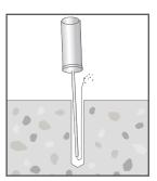
Blow out from the base of the drill hole at least 2 times until removed air is free of noticeable debris. For drill holes up to 18mm diameter - a manual blower pump may be used to clean the hole. For larger diameter holes - compressed air cleaning must be used for smaller holes.
