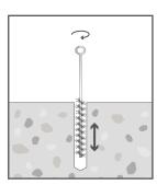
Brush 2 times with a wire brush (its diameter should be greater than the drill hole diameter) - inserting the brush to the base of the hole and withdrawing it with a twisting motion. If no resistance is felt during this step, the brush is worn - replace it.
