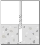
Drill hole into substrate to the specified diameter and depth using a rotary hammer drill and correctly sized carbide bit.
