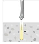
With the cartridge nozzle tip at the base of the cleaned drillhole,injectadhesiveuntil the hole is approximately 2/3 full. Slowly withdraw the nozzle from the hole whilst injecting, keeping the nozzle tipimmersed in the adhesive. This will avoid creating air pockets within the adhesive.
