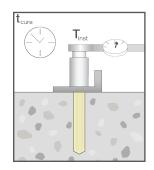
All steps prior must be completed within the working time of the adhesive. Protect the anchor from disturbance until the full curing time has been reached. Once full cure is achieved, carefully place the fixture and apply the specified installation torque.
