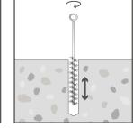
Brush 4 times with a wire brush (its diameter should be greater than the drill hole diameter) - inserting the brush to the base of the hole and withdrawing it with a twisting motion. If no resistance is felt during this step, the brush is worn replace it.
