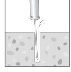
Blow out from the base of the drill hole at least 4 times until removed air is free of noticeable debris. For drill holes up to 22mm diameter - a manual blower pump may be used to clean the hole. For larger diameter holes - compressed air cleaning must be used and may also be used for smaller holes.
