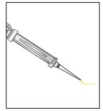
Prior to dispensing into the anchor hole, squeeze out a 10cm length bead of material and discard. The adhesive should now have a consistent, uniform color indicating correct mixing is occurring.
