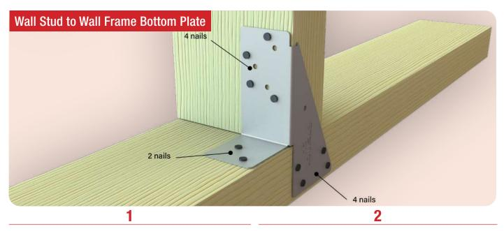
Locate the Bremick<sup>®</sup> Triple Grip into position. The vertical is sitting flush against the wall stud and the edge of the wall frame bottom plate. The folded flange is sitting on top of the wall frame bottom plate.
