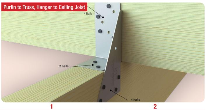
Locate the Bremick® Triple Grip into position. The vertical is sitting flush against the truss or hanger and the edge of the truss or ceiling joist. The folded flange is sitting on top of the truss or ceiling joist.
