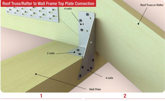
Locate the Bremick<sup>®</sup> Triple Grip into position. The vertical is sitting flush against the truss/rafter and the edge of the wall frame top plate. The folded flange is sitting on top of the top plate of the wall frame.
