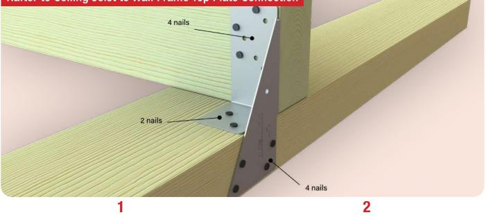
Locate the Bremick<sup>®</sup> Triple Grip into position. The vertical is sitting flush against the rafter or ceiling joist and the edge of the wall frame top plate. The folded flange is sitting on top of the top plate of the wall frame.
