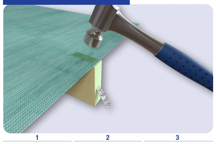
Place the Shade Fix approximately 5mm from the edge of the fabric or centrally on the timber batten.
