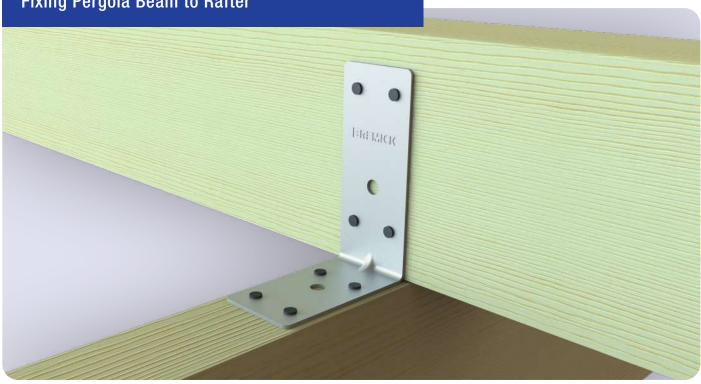
Locate the Bremick® Pergola Angle bracket, so the longest flange sits flush against the timber rafter face and the shortest flange runs along the top of the timber beam and is centrally located.
