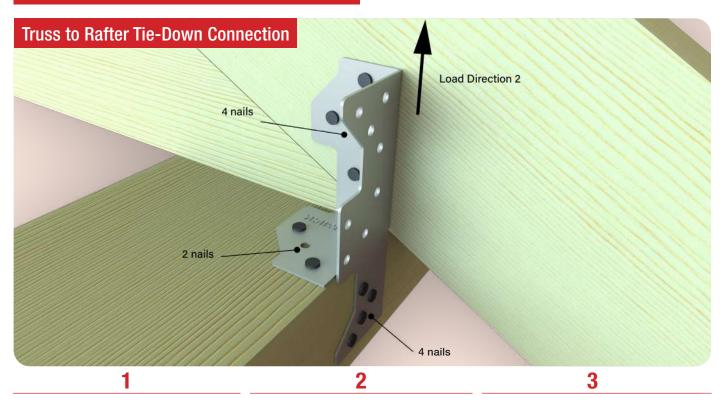
Fold up 1 flange of the Bremick® Multi Grip so it is sitting at right angles to the vertical. Locate the Bremick® Multi Grip into position. The vertical is sitting flush against the truss/ rafter and the folded flange is sitting on top of the supporting beam or top plate of the wall frame.
