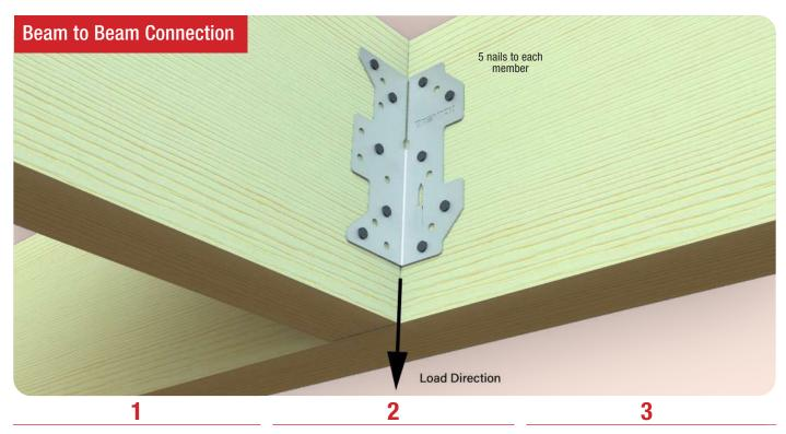
Locate the Bremick® Multi Grip into position, so each flange is flush against the 2 timber beams, that are at right angles to each other. Fix 5 x Bremick® Timber Connector Nails through the pre-punched holes into each timber member, as described in the image. Repeat steps 1 and 2 on the other side of the timber beam.
