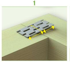
Locate the Bremick<sup>®</sup> Mini Nail into position. For butt joining, ensure an equal length on both sides of the joint.
