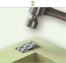
Install the Mini Nail by hammering on the top of the nail plate and ensure the plate is flush against the timber.
