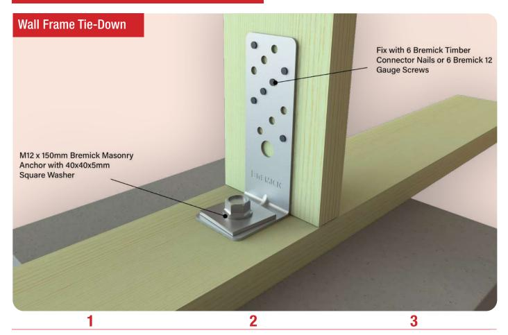
Locate the Bremick Hold Down Bracket, so the longest flange sits flush against the timber stud face and the shortest flange runs along the bottom plate of the wall frame and is centrally located.
