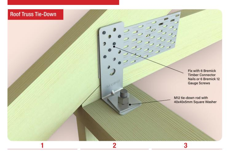
Prior to fixing the Bremick® Hold Down bracket, install the tie-down rod into the wall frame. Take into consideration that the rod will need to feed through the pre-drilled hole of the bracket.
