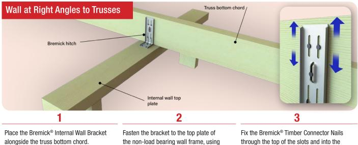
the non-load bearing wall frame, using Bremick<sup>®</sup> Timber Connector Nails. Locate the nails through all the pre-punched nail holes. Fix 3 nails in the base of the bracket. Fix the Bremick<sup>®</sup> Timber Connector Nails through the top of the slots and into the truss bottom chord. Ensure not to drive the nails fully home, as this will allow vertical movement of the truss. The nail should sit proud of the slots. 2 nails should be fastened into separate slots.
