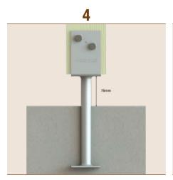
• Feed the 2 x M10/M12 bolts through the bolt holes and timber post. Locate washer and nuts onto the bolts and tighten. A minimum of 2 x thread pitch should extend beyond the outward surface of the nut.
