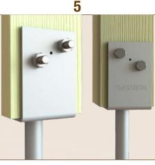
Alternatively install 18G x 45mm or 24G x 50mm construction screws through the bolt holes or M10/M12 coach screws.
