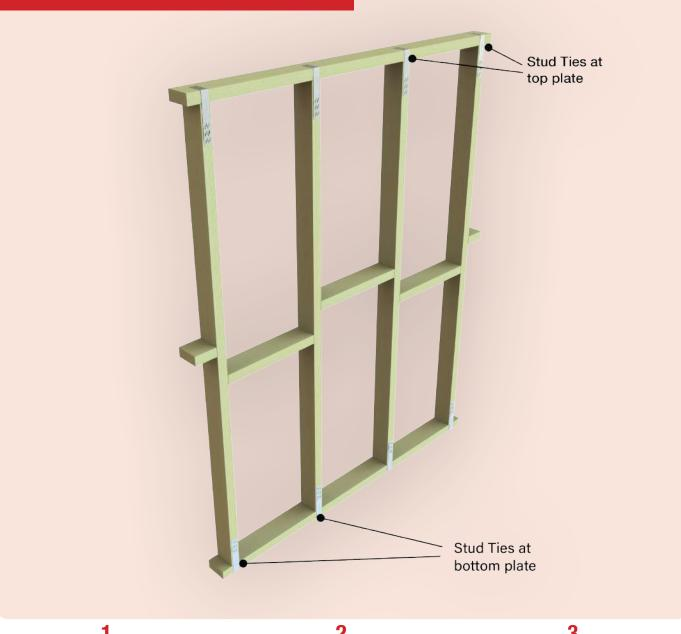
Locate the Bremick® Easy-Fix Stud Tie on the external corner of the top or bottom plate of the wall frame and centrally within the stud.
