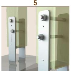
. Drill through the bolt holes located in the side of the post anchor to accommodate M12 bolts. Ensure the drilled holes are horizontally level and perpendicular to the saddle.
