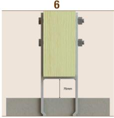
• Feed the 2 x M12 bolts through the bolt holes and timber post. Locate washer and nuts onto the bolts and tighten. A minimum of 2 x thread pitch should extend beyond the outward surface of the nut.
