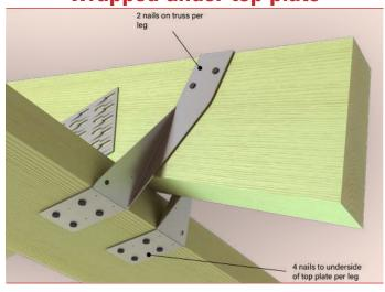
Use a hammer to fold the excess of each tie leg under the supporting member and secure each leg with 4 x Bremick® Timber Connector nails (or 5 x machine driven nails) to the underside.
