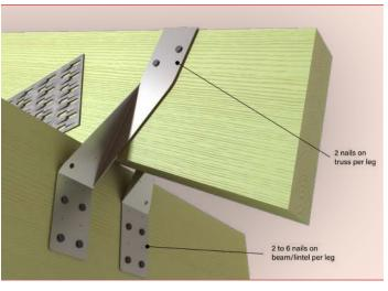
Fasten each leg of the Cyclone Tie to the face of the supporting member with 6 x Bremick® Timber Connector nails (or 8 x machine driven nails) to achieve the capacity.
