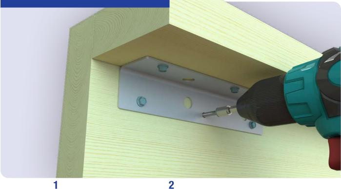
Fasten the flange of the Bremick<sup>®</sup> Heavy Duty Angle Bracket to the first timber member in the desired location and angle, by drilling Type 17, 12g x 35mm or 65mm timber screws through the 3 available screw holes.
